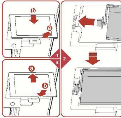
1. Open the back cover by (a) lifting cover and (b) sliding it out.
